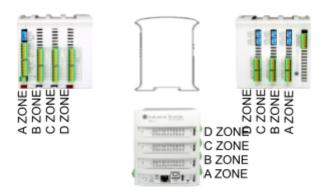
• The inputs in the A/B/C zones are named IX.X, being X any suitable number in the Shield. Outputs are named QX.X.
