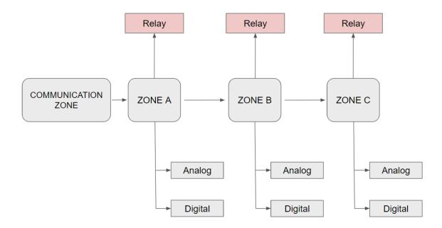
This is the possible zones scheme, whether the zone is Analog/Digital or Relay depends on your device model, which can be consulted on the <u>Zones Table</u>. The distribution of the different features provided by the ESP32 PLC Family are described below.
