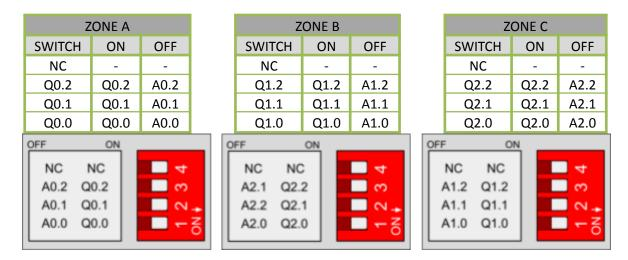
For the Analog Shield if a switch is set to ON, it can only act as Digital Output. If it is set to OFF, it can only act as an Analog Output.
