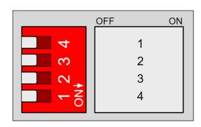
**RS484/Serial1/RS232/Serial2/EXP2:** This switch configuration can be done following the previous table to select among RS485 or Serial1 and RS232 or Serial2 or EXP2 (Expansion shield 2).
