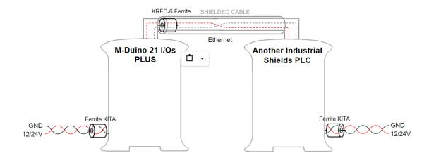
For Ethernet communication between two Industrial Shields equipment an **SFTP CAT-6 Ethernet crossover cable** must be used.
