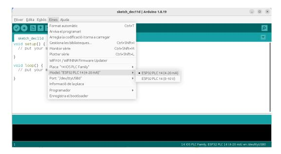
There, it is possible to select the mode used for the ESP32 PLC 14. In this case 14 IOs PLC (4-20 mA).
